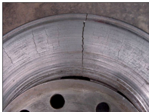
Defective rotor due to the appearance of cracks
