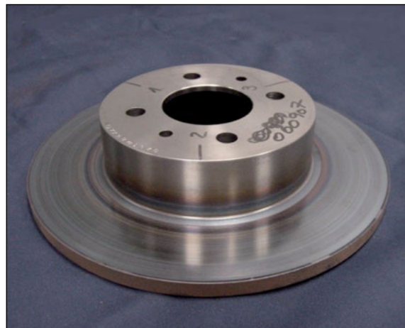
Defective rotor due to being subjected to excessive temperatures
