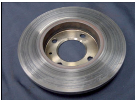
Defective rotor due to incorrect fitting of the calliper
