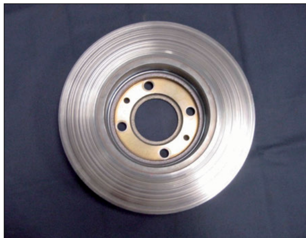
Defective rotor due to total wear of the pads
