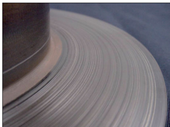
Defective rotors due to the generation of grooves and deep cracks
