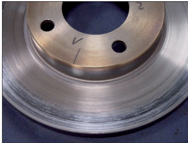
Defective rotor due to poor quality of the friction material
