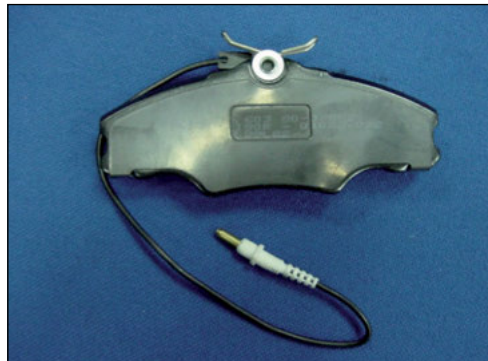
Pad with warning light
